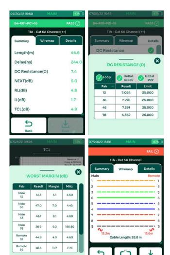
TestPro supports testing and certification for network deployments up to 40 Gigabit Ethernet for Cat3 through Cat8.2 or Class I/II cabling system. The electrically centered test plug assures the Level 2G/VI accuracy required to support field testing to Cat 8 / Class I/II, and actually exceeds the 2000 MHz requirement, to offer a 3000 MHz platform. The 3000 MHz frequency range provides investment protection as standards evolve, the test platform is ready.
